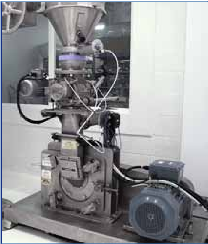
This Mobile Kek Universal Mill system improves flexibility and is easily relocated between production areas.
