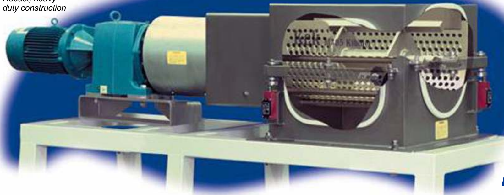
Cantilever Shaft Kibbler with no end bearings
