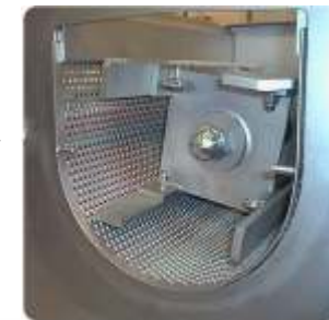
Cantilever Shaft Kibbler with no end bearings
