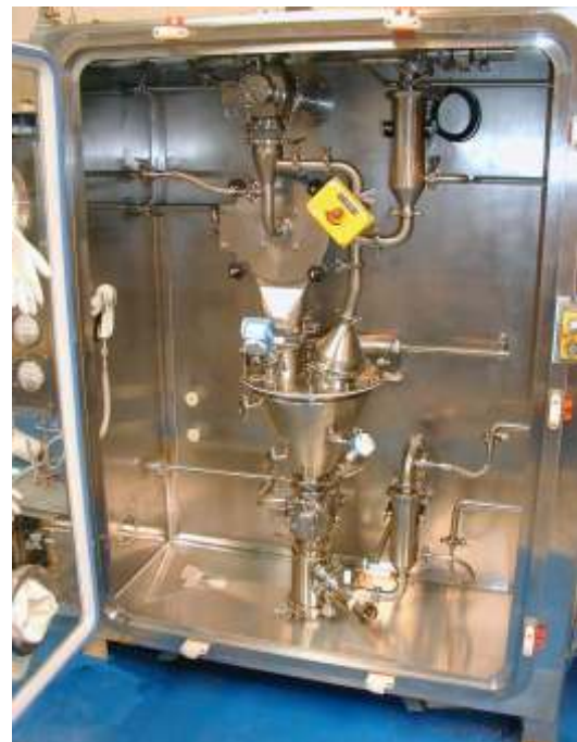
A pharmaceutical pilot scale Pin Mill in a glove box isolator
