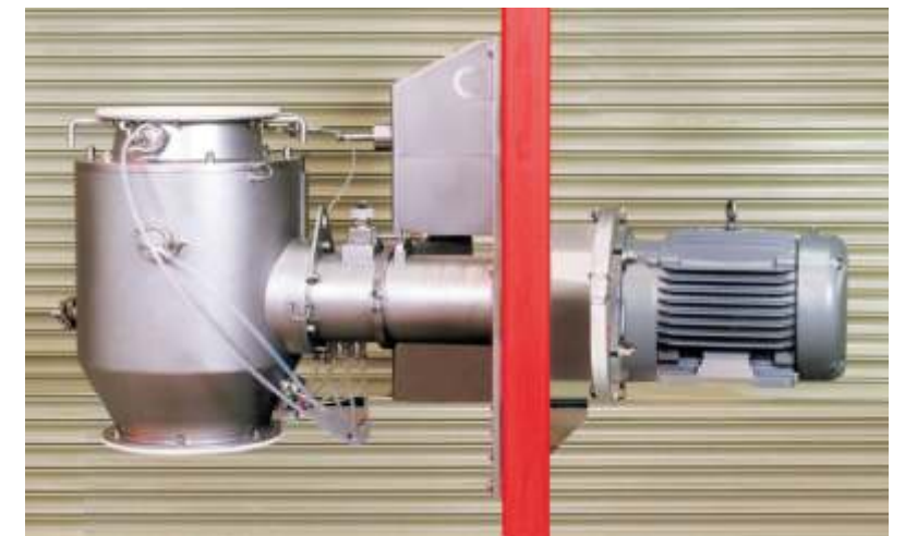
A Kek 340 Cone Mill with 'thru-the-wall' drive
